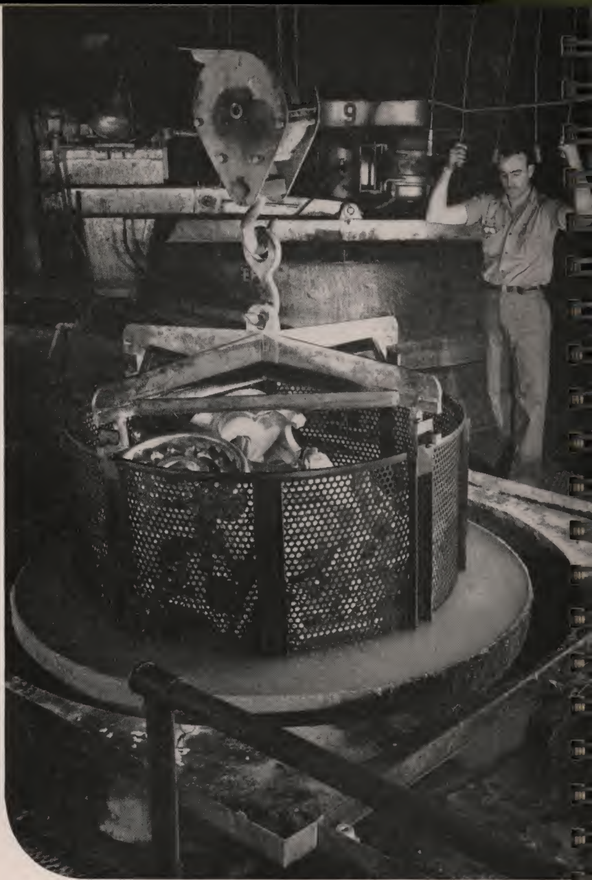
Lowering a basket of aluminum forgings into a quenching tank, after heat treatment.
